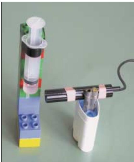
**Fig. 1. Water-drop projector: experiment setup.**
