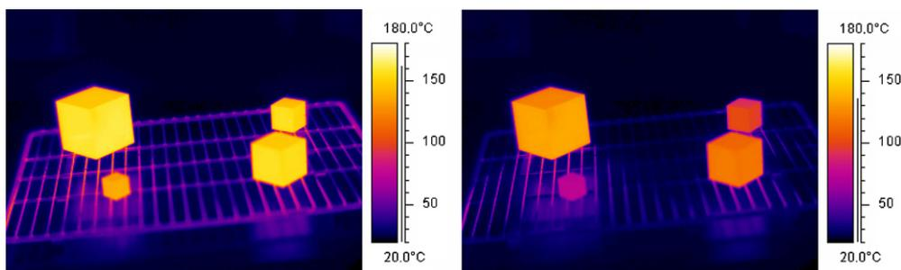
**Figure 8.** IR images of four aluminium cubes of 20 mm, 30 mm, 40 mm and 60 mm length near the beginning (left) and during the cooling process (right). Small cubes cool down fastest.
