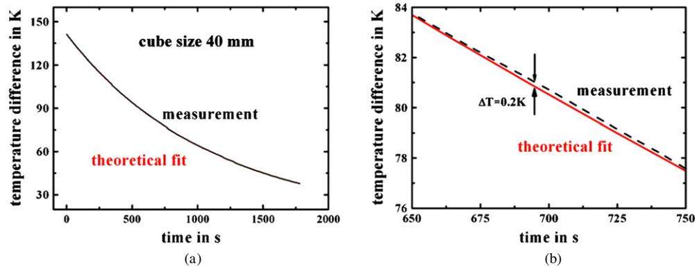
**Figure 10.** (a) Comparison of experimental cooling curve with the theoretical prediction of an exponential law given by (12). The agreement of the experiment with the exponential law is very good, even in the magnified part of the plot (b).
