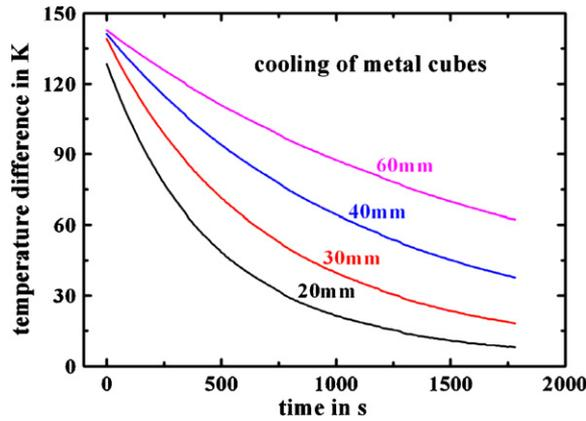
**Figure 9.** Measured temperatures during the cooling curves of metal cubes from figure 8, detected with IR imaging.
