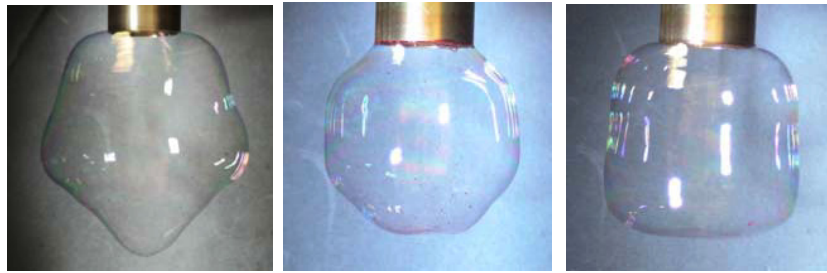
Figure A1. Results of students' project: three modes of oscillation of soap bubble (project number 1).
