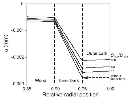
Figure 4. Field of radial displacement ( $u$ ) at the tree periphery, computed for various values of the ratio of outer bark to inner bark stiffness  $C_{TT,4}/C_{RR,3} = 10, 50$  or  $100$ .
