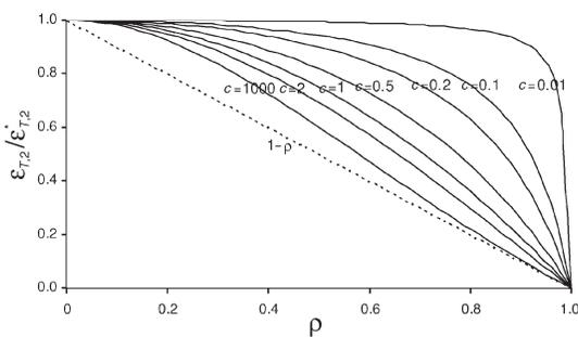
Figure 2. Reduction in apparent strain in response to an inner core of nonconducting tissue for various relative thicknesses of this core ( $\rho$ ) and stiffness ratios ( $c$ ).
